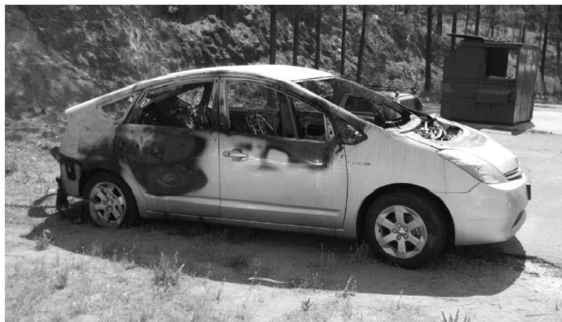
Figure 1.5 Remains of a Prius PHEV after its Li-Ion traction pack caught fire.
